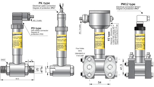
Transmitter HDPM-40 Process connection GP type Static pressure limit 40 bar
