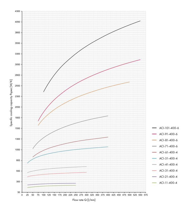
The specific cooling capacity indicated in the graph was determined on the test bench, test oil ISO VG 46, oil-inlet temperature 60°C. The actual cooling capacity may deviate by approx. ± 5 % depending on the installation site and other operating parameters.
