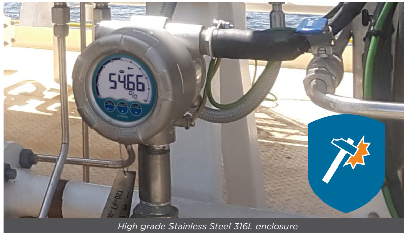
High grade Stainless Steel 316L enclosure
