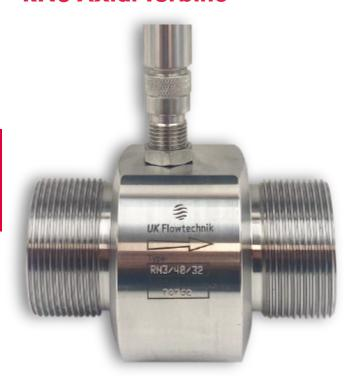
The RN3 series axial turbine flow meter is used for liquids such as water, light oils, solvents (such as methanol) and low viscosity chemicals in applications such as batching, flow rate monitoring, controlling, blending and filling. The RN3 is highly accurate and often used for testing the performance of pumps, engines, valves and other flowmeters. In hazardous areas you can use the flowmeters with the Intrinsically Safe of Flame Proof pick-off coil with options for directly mounted displays.
