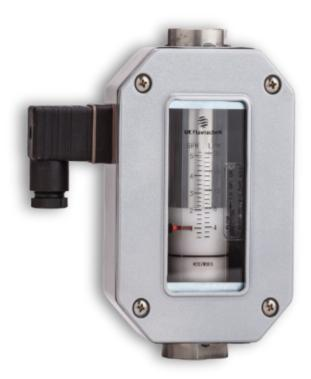
The M & N Series offer the same versatility as the B Series meter with the addition of one or two flow alarms in the form microswitches. This makes them ideal to provide a low flow cut-off to protect a hydraulic or cooling water pumps and bearing lubrication/cooling water circuits to prevent damage. With pressure ratings up to 414 Bar even jacking circuits for hydrodynamic bearings can be monitored. The air/gas scales also mean they can be used to detect compressor and Nitrogen blanket failures.
