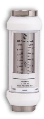
For higher temperature applications such as thermal or heat transfer fluids, high performance gear boxes and boilers the H & J Series provides an in-line solution for direct reading of the flow rate without any additional powered requirements. They offer the simplicity of the B Series and by using special materials such as PTFE and Pyrex can withstand fluid temperatures of up to 315oC.
